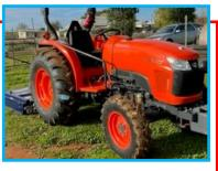
vehicle to learn and further develop their skills in tractor use and driving. The tractor came complete with a PTO and 3-point linkage rotary hoe and slasher. These implements are important for use in learning about PTO safety. Keep an eye out for the bright orange tractor being put to use around the ag plot and farm.
